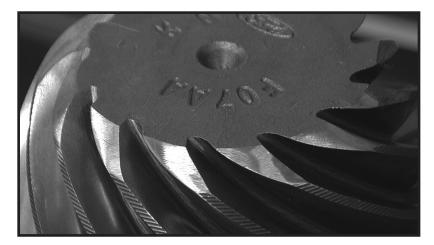
This modification of the pinion head will not affect its performance or strength. The area you will be removing is usually well outside the contact pattern.
