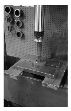
Use the press to gently push the axle down to safely and easily remove the bearing.
