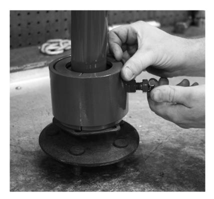
Slide the retaining sleeve over the clamshells. Tighten down the retaining bolt to secure the retainer and clamshells in place.
