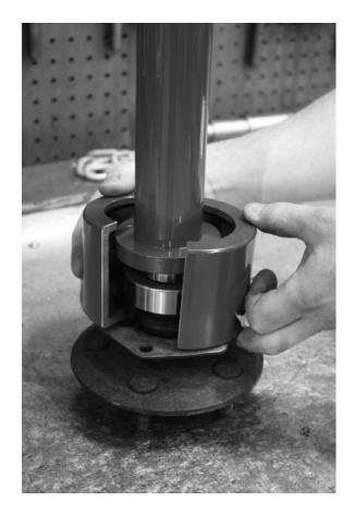
Place the clamshells on the puller and axle. The bottom of the clamshells goes under the axle bearing. The top of the clamshells should clear the lower lip of the puller.
