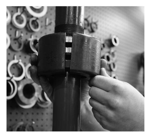
Once seated against the body of the axle bearing puller, place the clamshells on the tools as shown.
