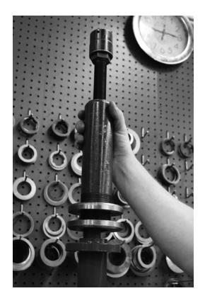
If using the axle bearing puller with a Yukon® carrier bearing puller, place the carrier bearing puller body over the top of the axle.
