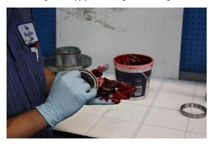
• Install the packed inner wheel bearing into the wheel hub.
