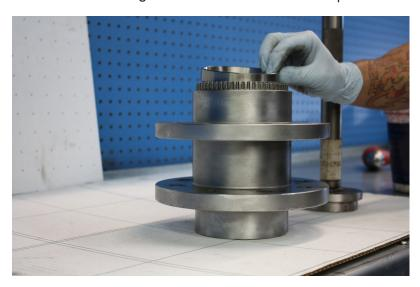
• Make sure bearing races are fully seated into the hub.
