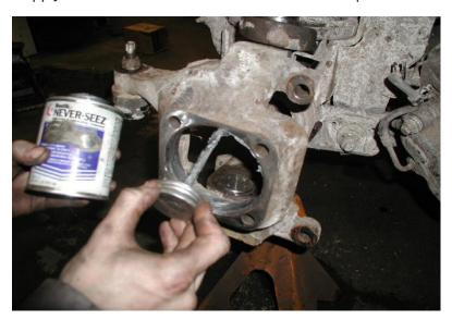
• Install the new spindle over the axle and into the steering knuckle. The 2 threaded holes must be aligned to the top of the steering knuckle. OEM dust shields must be located between the steering knuckle and the new spindles. Torque supplied hardware to 135 ft/lbs.
