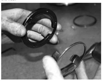
11. Install the hub snap ring into the hub. A small amount of force may be necessary to compress the cam spacer into the hub to allow extra clearance for snap ring installation. Be sure snap ring is fully seated into the snap ring groove of the hub.
