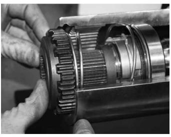
9. While fully compressing the assembly install the axle snap ring if applicable. Assure the snap ring fully seats into the groove on the outer shaft. If no outer snap ring groove exists proceed to the next step in assembly.
