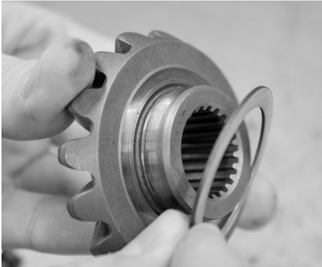
Figure 3 - MUST REMOVE thrust washers
